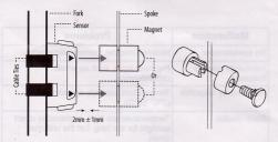
Attach the sensor transmitter to either front fork using the supplied cable ties. Fit the magnet to a spoke using the diagram above as a guide. Position the sensor & magnet as shown above. Take care to align the magnet to either arrow on the sensor with  $2\text{mm}\pm1\text{mm}$  gap in between.
